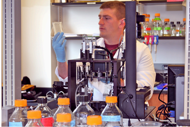
Graduate Student Jason Westerbeck Examining Yeast Colonies Arrayed on a Media Plate by the Norgren CP7200 Colony Picking Robot.
